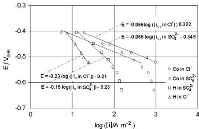
**Fig. 6** Tafel plots for deposition of cobalt and evolution of hydrogen in chloride and sulphate electrolytes (see Tables 4 and 5)
